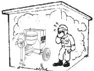
flow is restricted it will cause serious damage to the mixer or engine and may cause injury to people and property. Remember the mixer's engine (gasoline models only) gives off **DEADLY** gases.
